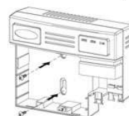
Step 3. Tighten the suitable screws which can support the weight of this unit securely.
